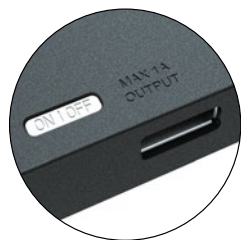
Optionally possible to charge the battery either via pad or USB port
